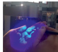
Example for pre-curing composites with the UV-light for a further elaboration
